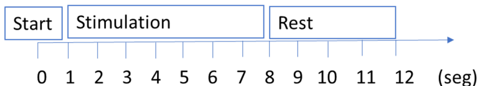
Figure 3. Timing of a single SSVEP trial.
