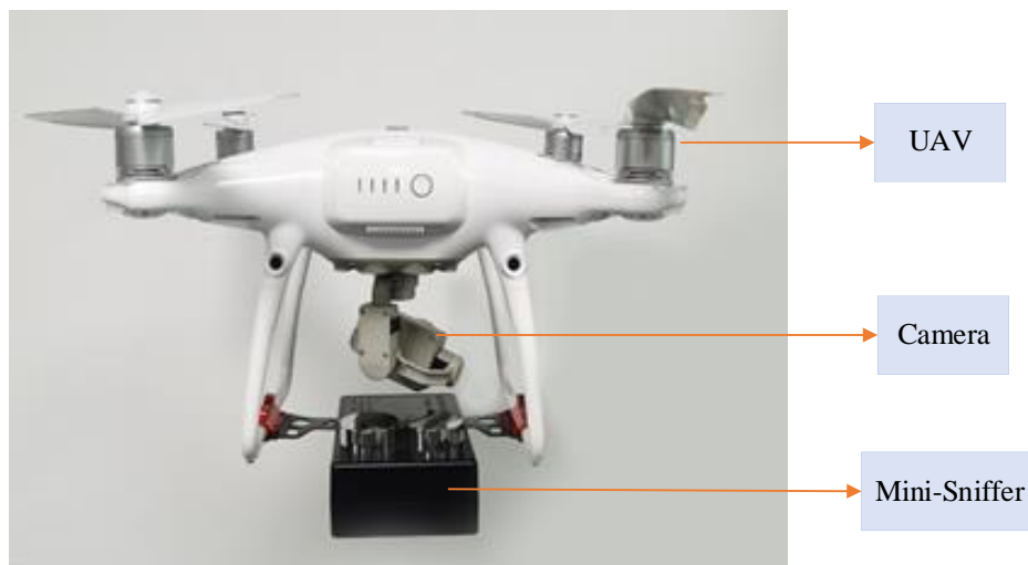
Figure 2. Image of ship exhaust mini-sniffing UAV system.
