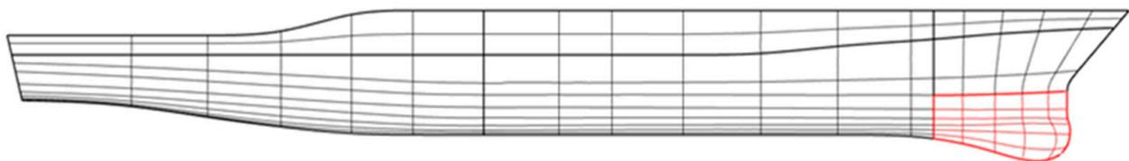
**Figure 1.** Ship model (side view). The red lines indicate the sonar dome.
