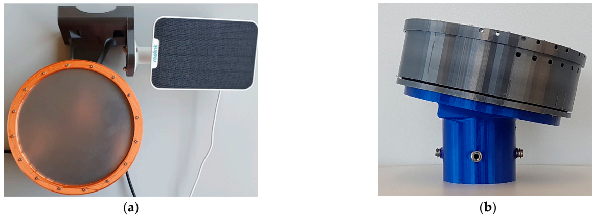
Figure 8. (a) Top view of the sensor with solar module; (b) Side view of the sensor with 25^\circ inclined mounting base.
