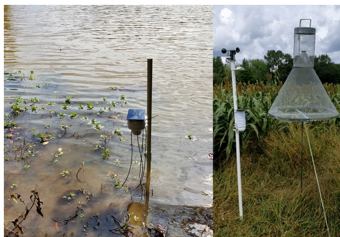
Figure 1. The system as deployed to measure bivalve activity (left) and moth activity (right).
