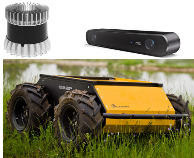
Figure 1. Photographs of an Ouster OS1-64 LiDAR ( up-left ), a ZED-2 stereo camera ( up-right ) and a Clearpath Husky UGV ( down ).
