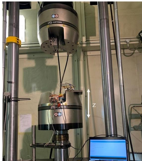
**Figure 4.** Laboratory validation of LARA: (a) mounting CHEAP and LARA to the shaking part of the jack, and (b) the used vibrating platform (INSTRON 8803).
