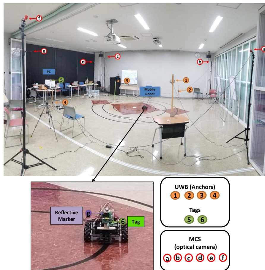
Figure 3. Position measurement system of IMU/UWB and MCS using a mobile robot.
