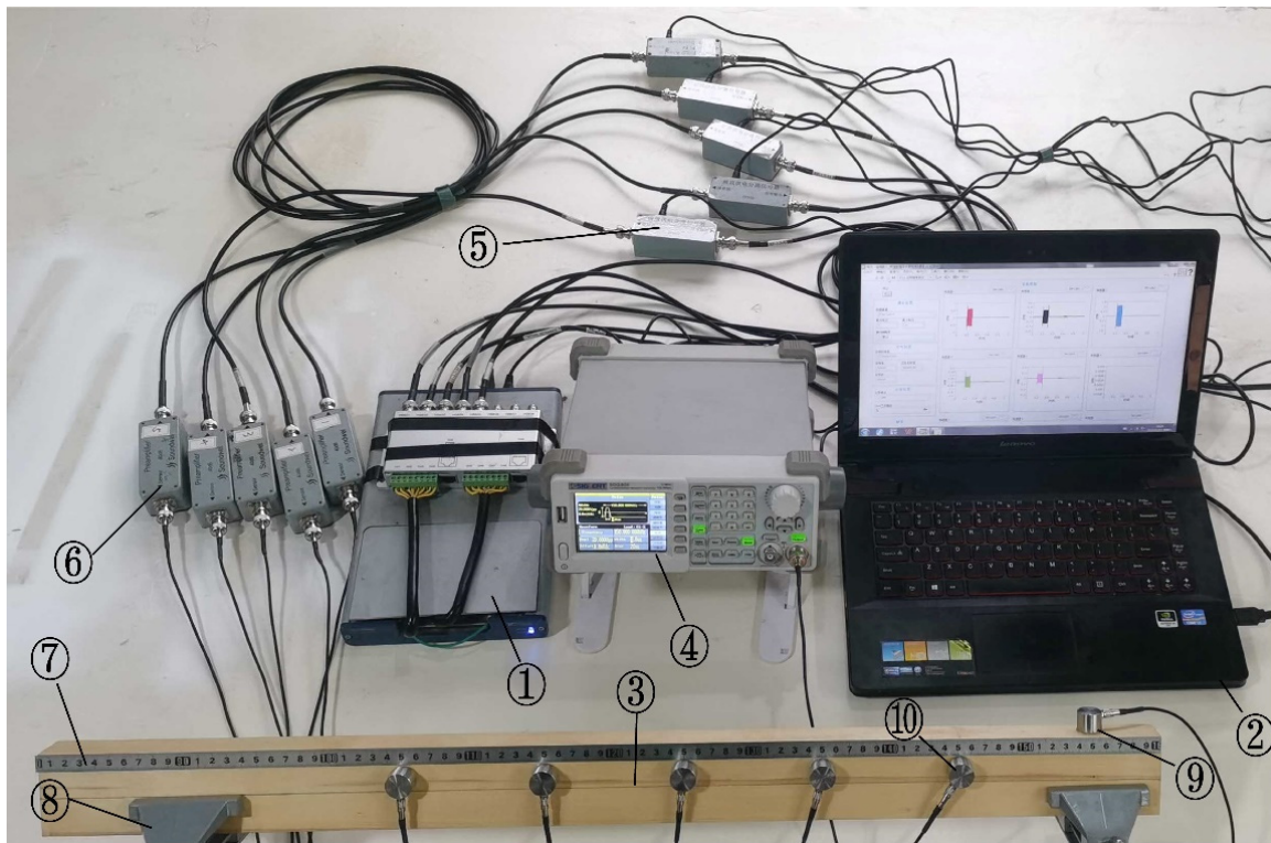
Figure 2. Test diagram. ① NI acquisition card ② Computer ③ Test piece ④ Arbitrary waveform generator ⑤ Signal separator ⑥ Gain amplifier ⑦ Scale ⑧ Table clamp ⑨ AE source ⑩ Sensor.
