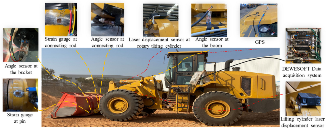
Figure 6. The layout of the sensors installed on the wheel loader.
