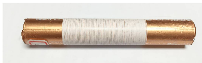
Figure 4. PVDF fibers collected by the hollow copper cylinder.
