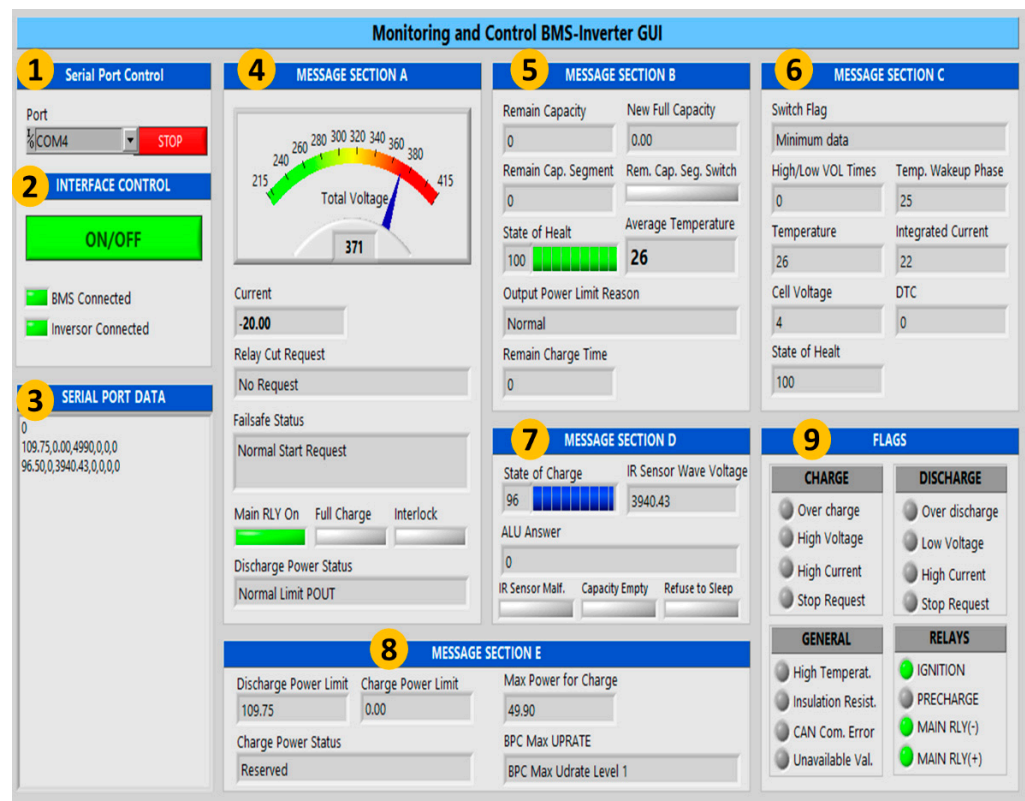
Figure 8. Monitoring and control BMS inverter GUI.
