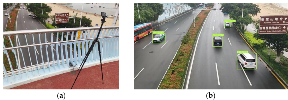
Figure 14. (a) Camera on pedestrian overpass. (b) Detection of vehicles in field measurement.
