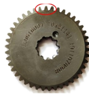
(b) Multitooth wear of planetary gear
