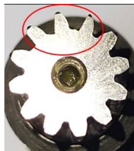
(a) Multitooth wear of sun gear
