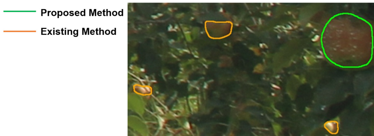
Figure 11. Example of small fruit detection. The proposed model outperformed the COCO learning model in mean and median IoU because it could accurately detect hidden regions of fruit without detecting parts of the fruit. The orange line is the result of the COCO as an existing method, and the green line is the result of the proposed method.
