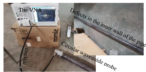
Figure 15. Experimental platform for small-diameter pipeline inspection.
