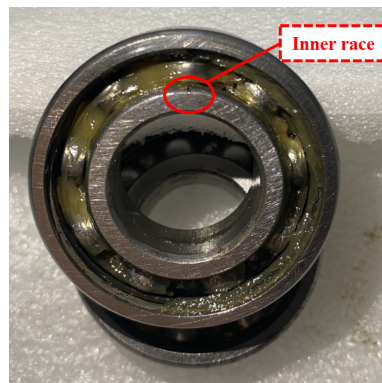
Figure 10. The test bearing with inner race fault.
