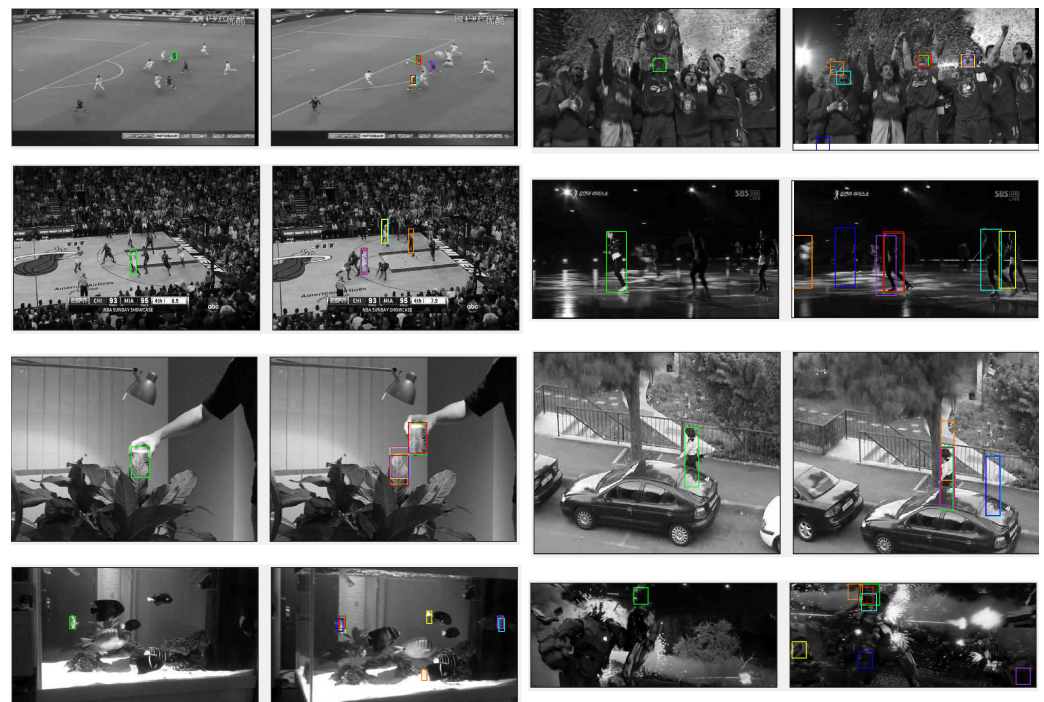
Figure 6. Comparison performance of different methods using the proposed feature extraction method. The colour boxes indicate the template location defined by: — Ground truth — BBS — CoTM — DDIS — DIM — NCC — QATM — SSD — ZNCC. Note that the colour images have been converted to greyscale in order to make the bounding boxes more visible. The boxes predicted by ZNCC and NCC are remarkably similar, and thus overlap.
