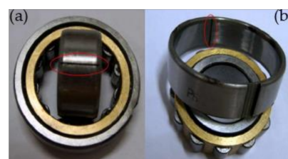
Figure 12. Type of rolling bearing failure. (a) is the inner-ring defect, (b) is the outer-ring defect.
