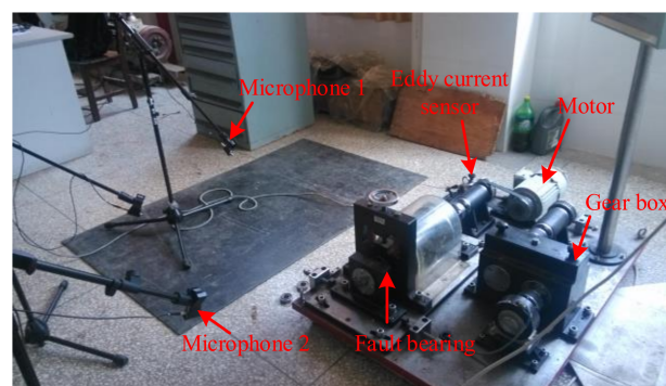
Figure 11. The layout of the test bench and microphone.
