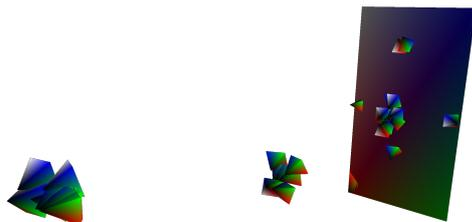
**Figure A1.** Visualization of camera poses for the dataset 0. The rectangle indicates the coding screen and each pyramid denotes a calibration camera pose. The projection center corresponds to the tip of each pyramid.
