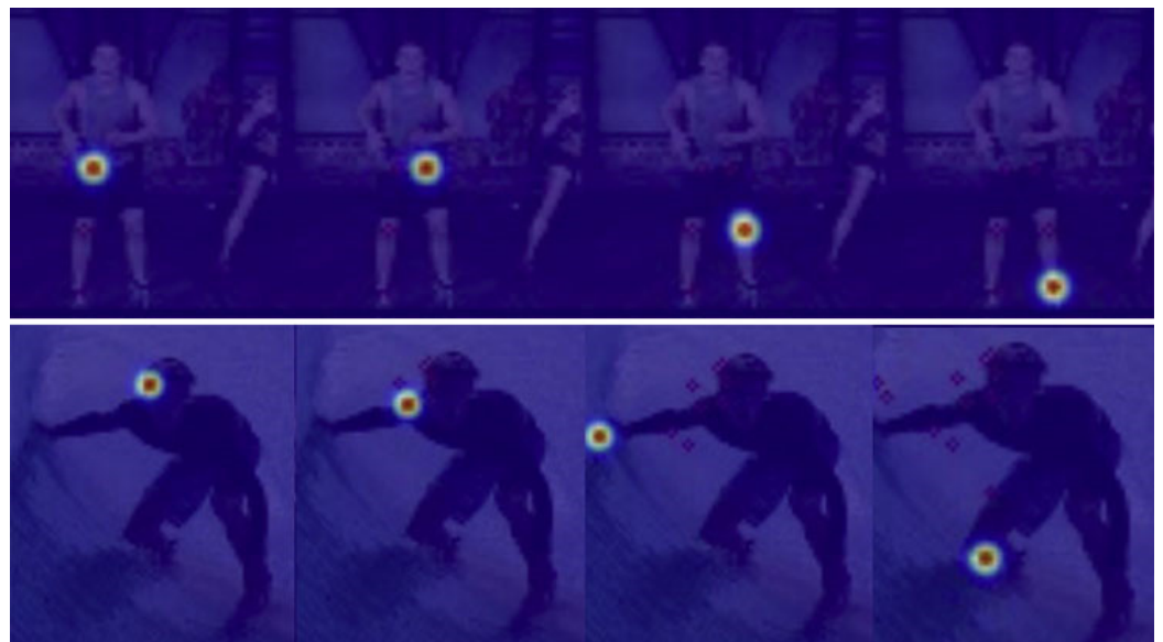
Figure 3. Visualization of Cofopose's process of decoding for the keypoint detection transformer on MPII and COCO is denoted by the first and second rows, respectively. For MPII, the first, second, third, and fourth columns represent the right hip, left hip, left knee, and left ankle, respectively. For COCO, the first, second, third, and fourth columns represent right eye, right shoulder, right wrist, and right knee, respectively.
