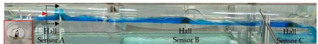
Figure 3. Experimental equipment of miniaturized subsea pipeline with hall sensors.
