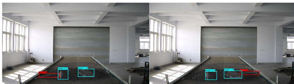
Figure 27. Semi-buried bolt and gangue detection.
