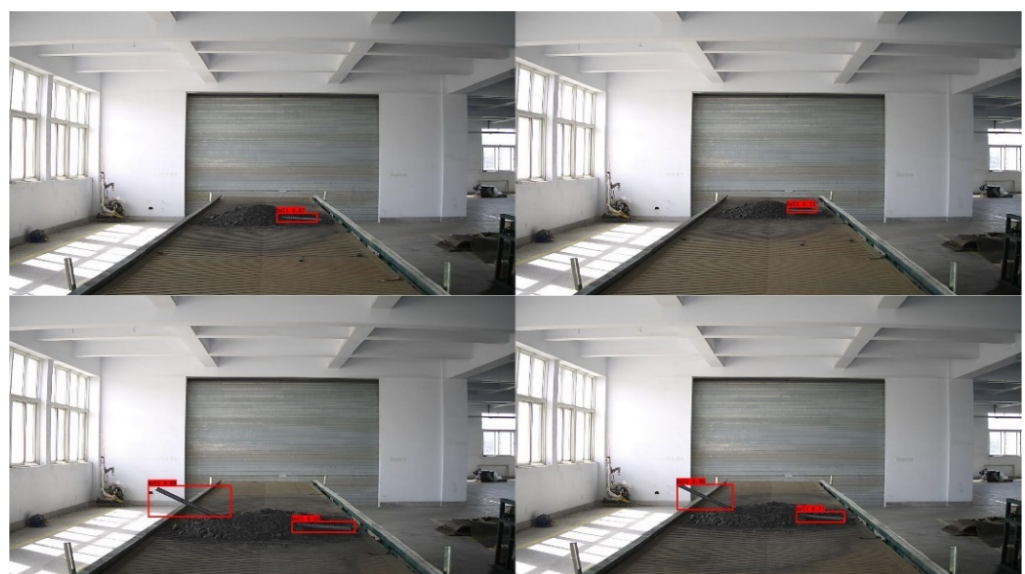
Figure 25. Semi-buried bolt detection.
