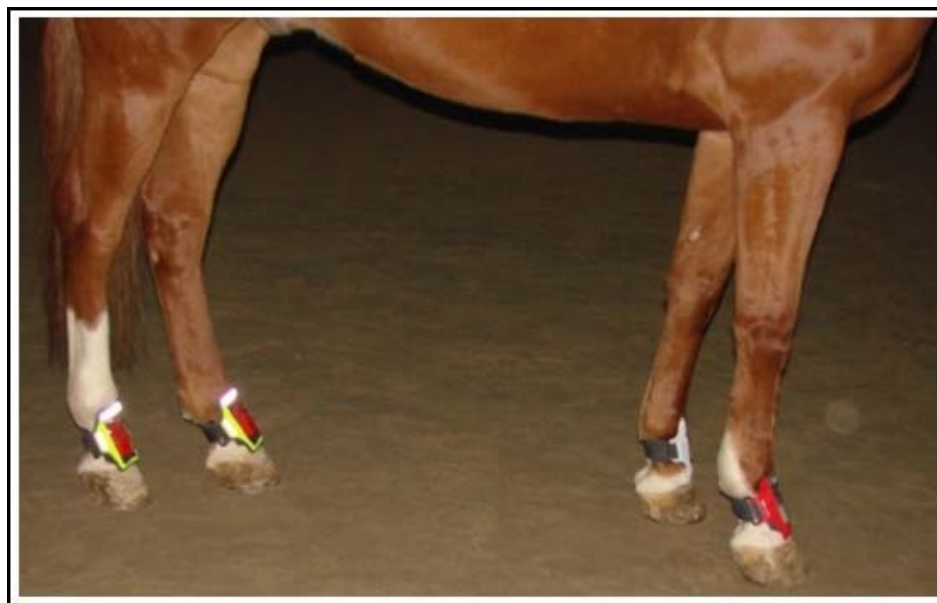
Figure 3. Illustration of correct fitting of the Lameness Detector 0.1 system with adjustable straps to the dorsal aspect of a horse's pasterns.
