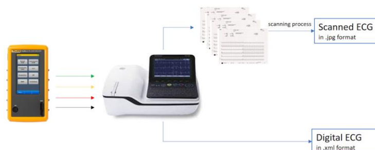
Figure 1. Data acquisition system. The scanning process is done by the Kyocera TASKalfa 5053ci scanner.
