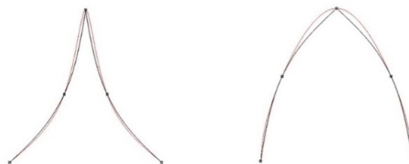
Figure 10. Undulations of the spline in the vicinity of kink point of curves making concave and convex connections.
