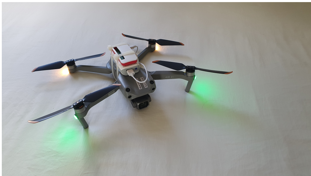
Figure 8. Drone attached to the Raspberry Pi Zero 2W.
