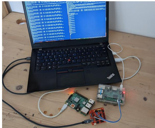
**Figure 4.** Testbed composed of a Raspberry PI 3B acting as the publisher connected to a laptop via a UART adapter that hosts the MQTT broker, a Raspberry Pi B+ acting as the subscriber.
