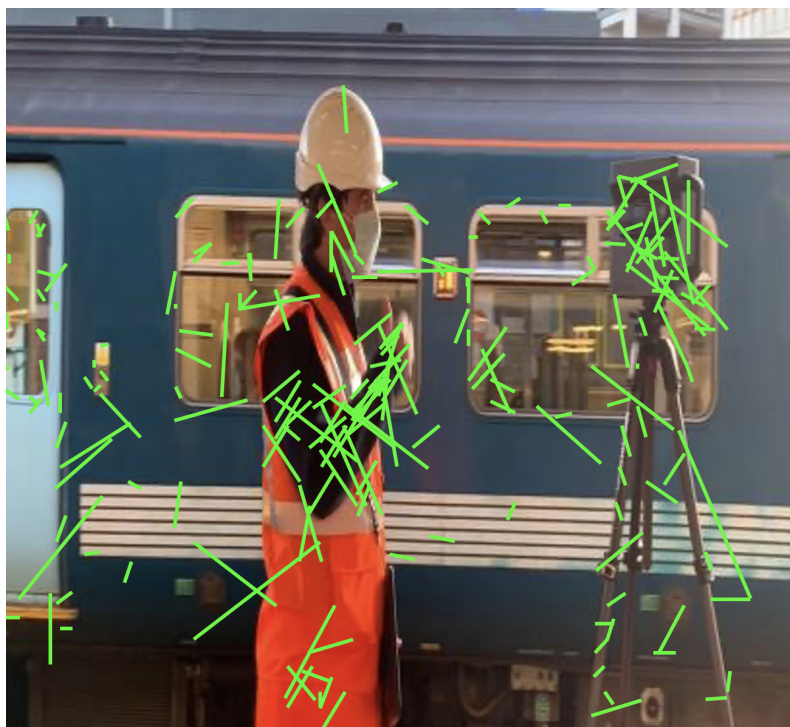
Figure 9. Experimental results of Lucas Kanade Optical flow method. Optical flow at high or normal wavelength is represented by the green line, while optical flow at low wavelength is represented by the green point.
