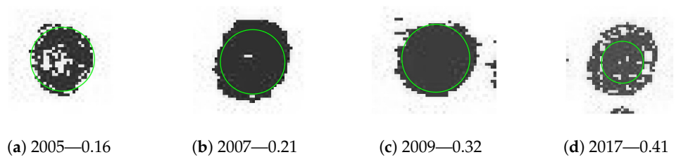
Figure A7. Case 2: the extracted grayscale images for the selected rivet with the feature values obtained for this rivet for subsequent years of inspection.
