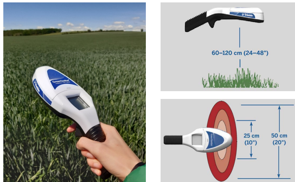
Figure 1. (Left) GreenSeeker spectrometer for ground measurements (photo: Paulina Raeva), (right) functionalities during NDVI field measurements.
