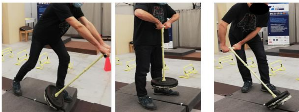
Figure 3. Example movements of the three motions that subjects were asked to perform in order to lift the mass: (left) pushing the pole, (middle) snatching the pole, and (right) pulling the pole.
