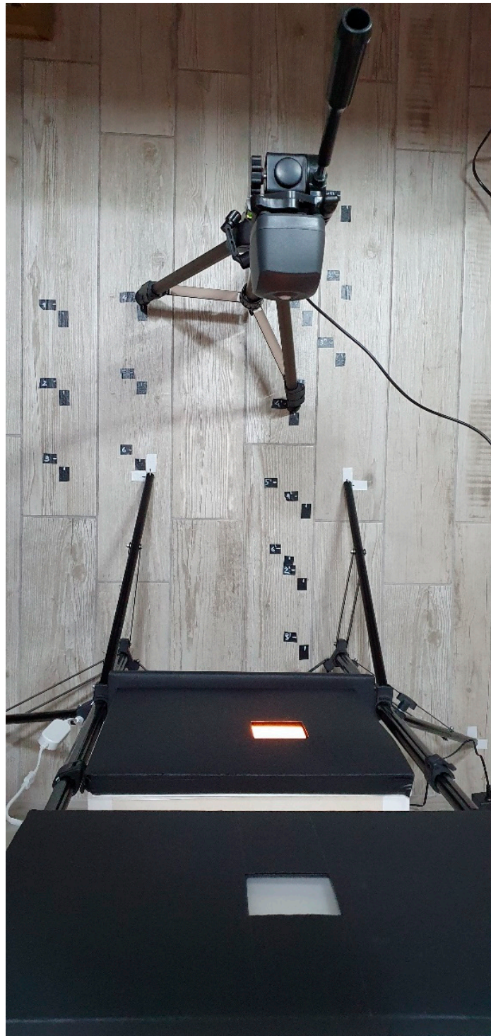
Figure 5. Plan view of the setup for acquiring the luminance mapping of the selected region of the LED panel and cube panel.
