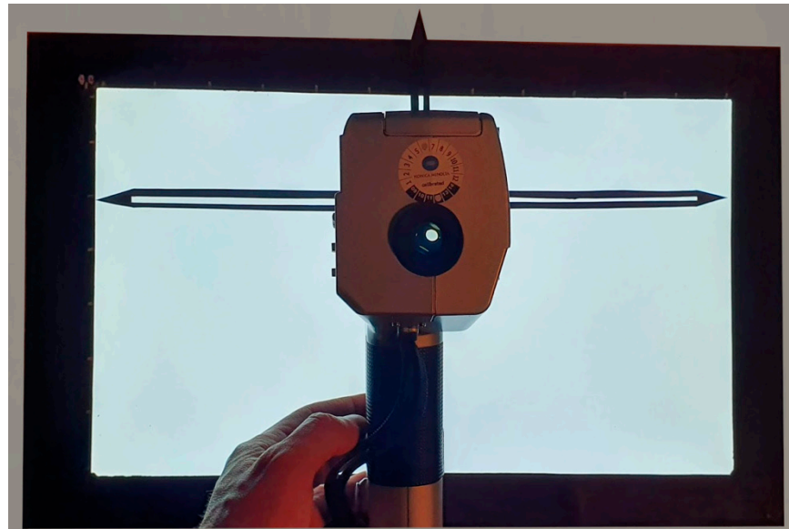
Figure 2. Example of characterisation of the LED panel (the same approach was used to characterise the cube).
