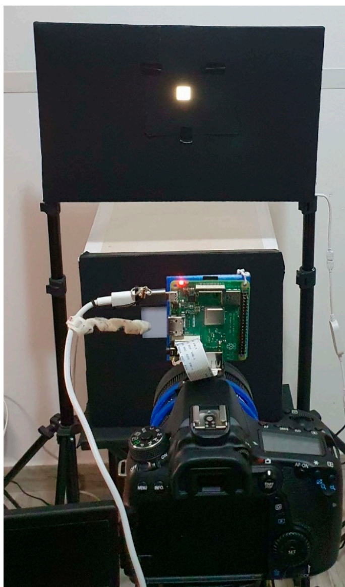
Figure 6. Setup for vignetting assessment: LED panel set as neutral white with 100% of intensity. Illuminated area = 2 \times 2 cm 2 . Low-cost camera positioned at 60 cm from the LED panel.
