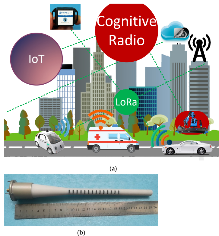
Figure 1. (a) Application areas of proposed antenna (b) Fabricated prototype of Embedded Helix and dielectric rod antenna.
