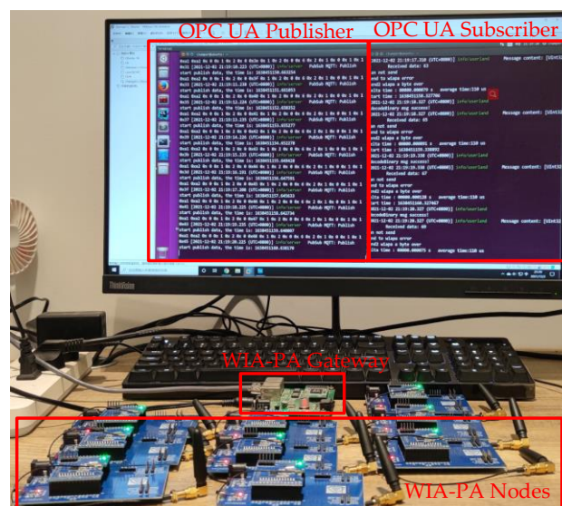
Figure 12. WIA-PA/OPC UA joint pub/sub experimental verification system.
