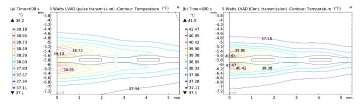
**Figure 14.** Contour plots of thermal analysis: (**a**) pulsed and (**b**) continuous transmission modes for 5 W LVAD.
