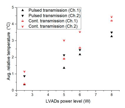
**Figure 10.** Average relative temperature change ( $\Delta$ T) in the subcutaneous tissues vs. power delivered to the load in pulsed and continuous transmission protocols from the in vivo measurements with power levels of 2.5 W, 5 W, 6 W, and 8 W.
