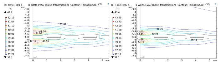
**Figure 15.** Contour plots of thermal analysis: (**a**) pulsed and (**b**) continuous transmission modes for 8 W LVAD.
