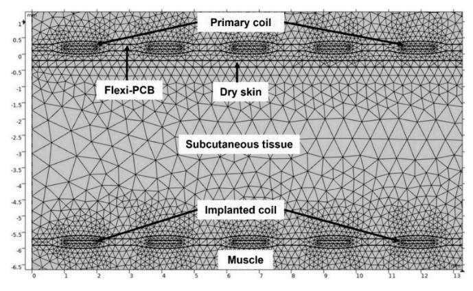
Figure 6. The geometry after applying the meshes.
