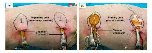
**Figure 4.** An in vivo measurement setup: (**a**) implanted coils underneath the skin, and (**b**) primary coils adhered above the skin.
