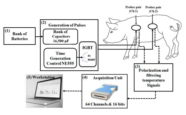
Figure 1. Schematic block diagram of the PLE system.
