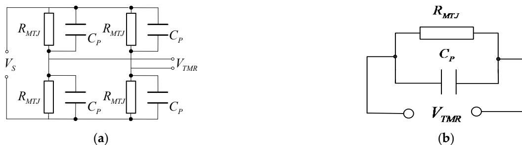
Figure 4. Structure of the TMR sensor. (a) Internal parasitic capacitance of the TMR sensor, (b) internal equivalent structure of the TMR sensor.
