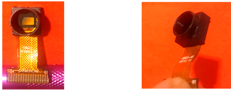
Figure 6. Lens seat with a ribbon connector. The image sensor can be seen from the left panel.
