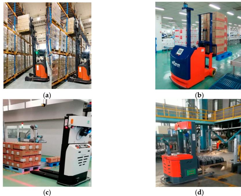
**Figure 1.** The specific pallet detection scene for automated guided vehicles. (a) Storage shelves, (b) the production workshop, (c) drug transport and (d) blast furnace conditions.
