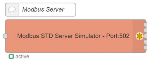
Figure 7. Node-RED Modbus server flow simulates the PLC.
