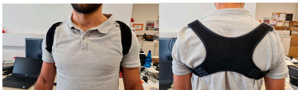
Figure 7. Second smart harness solution positioning SWs on shoulders and back.
