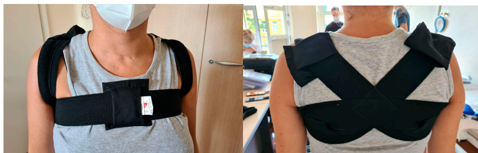
Figure 6. First smart harness solution positioning SWs on shoulders and chest.
