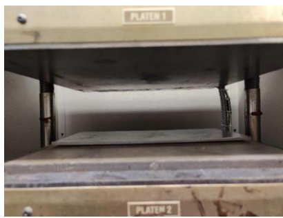
(a) – View of hot press top-bottom platens (Actual)
