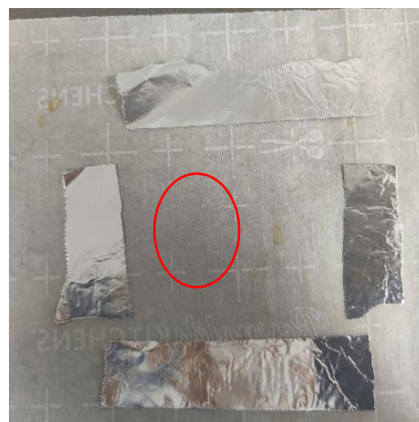
Figure 15. One 114 kGy PLA resin bead compressed under 6228 N, 193 °C/12 min. Remnant PLA resin almost invisible (encircled).
