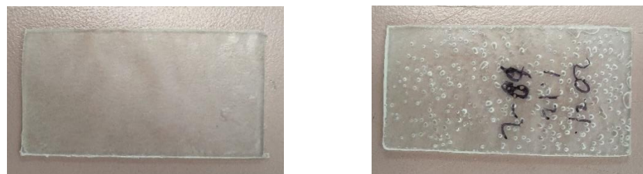
Figure 14. MLR experimentation samples. Left: control (0 kGy)-no visible pores; Right: 56 kGy gamma dose pre-irradiated—showing visible pores.
