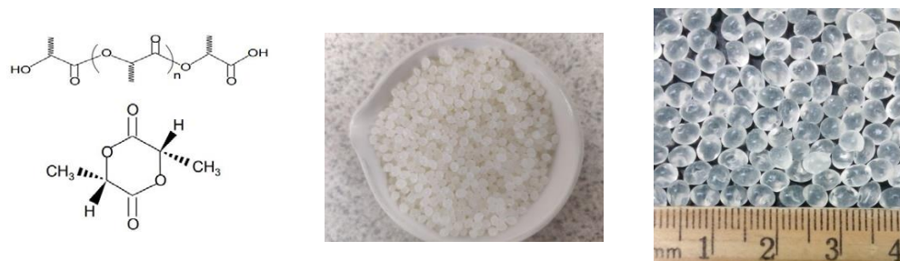
Figure 1. PLA molecular structure, ~3 mm resin beads in cup and closeup with scale—PLA resin supplied by Natureworks, LLC.
