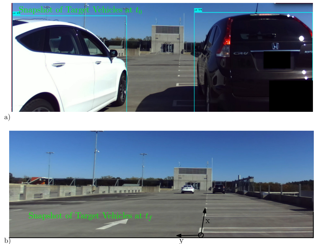
Figure 16. Experimental setup for the case of multiple ET target tracking scenario. (a) The target vehicles ( ET_1 (Sedan Car), ET_2 (SUV Car)) are pictured at the starting pose t = t_0 . The rover station of the RTK GPS is placed at the center of the rear axle of ET_1 (Sedan Car). (b) The time-snapshot of both target vehicles is shown at t = t_f . The positive x-y coordinate axes of the radar sensor are also depicted.
