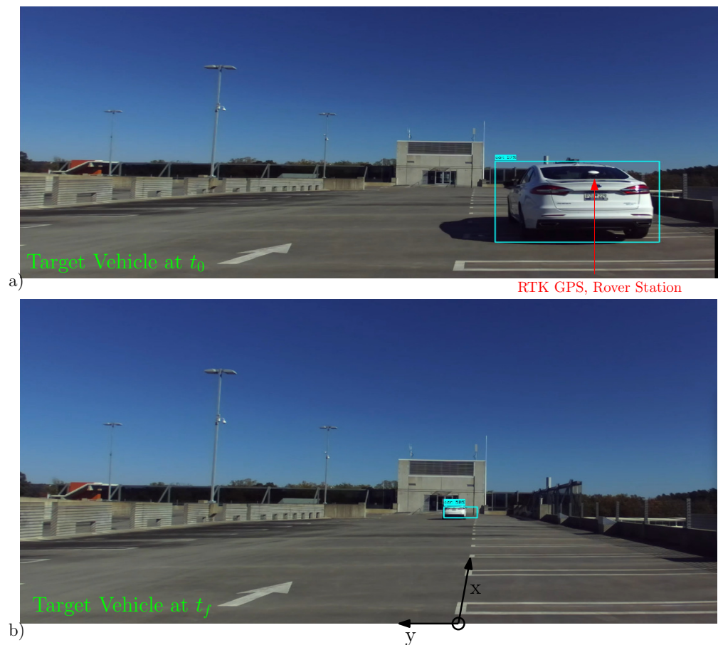
Figure 12. Pictured here is the experimental setup for a single target tracking scenario. (a) The target vehicle is shown at its starting pose at t_0 . The rover station of the RTK GPS is also shown positioned at approximately the center of the rear axle. (b) The target vehicle is shown positioned at t = t_f . The positive x-y coordinate axes of the radar are also depicted.
