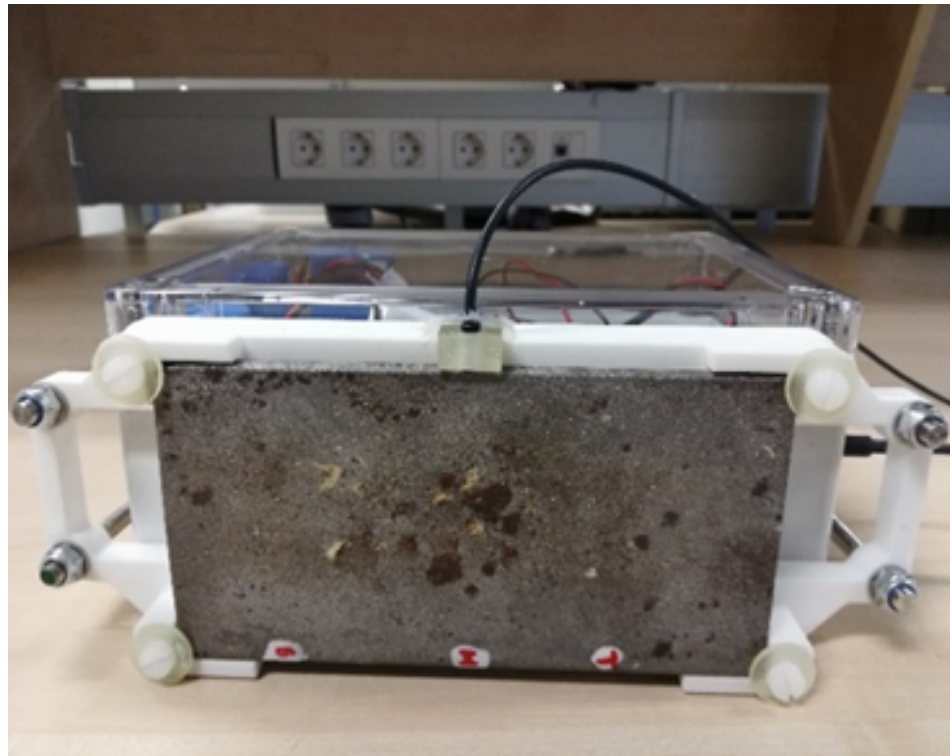
Figure 9. Bare steel sample attached to the monitoring solution.
