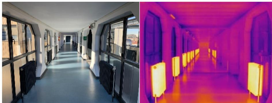
**Figure 7.** Visual (left) and thermal (right) images of the indoor environment used to test the proposed algorithm. Notice how the thermally distinctive elements on both sides of the corridor are still recognizable in the thermal scene (Figure 8) as well as in the corresponding temperature maps (Figure 9a,b).
