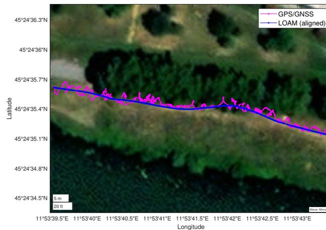
**Figure 13.** Comparison between the trajectory reconstructed in real-time using the *livox\_horizon\_loam* algorithm (blue) and the path traced by the rover's GPS/GNSS receiver (purple). Here the Horn's quaternion-based algorithm was used to align the two paths and to represent the reconstructed trajectory in the same latitude/longitude/altitude coordinate system used for the GPS/GNSS points.
