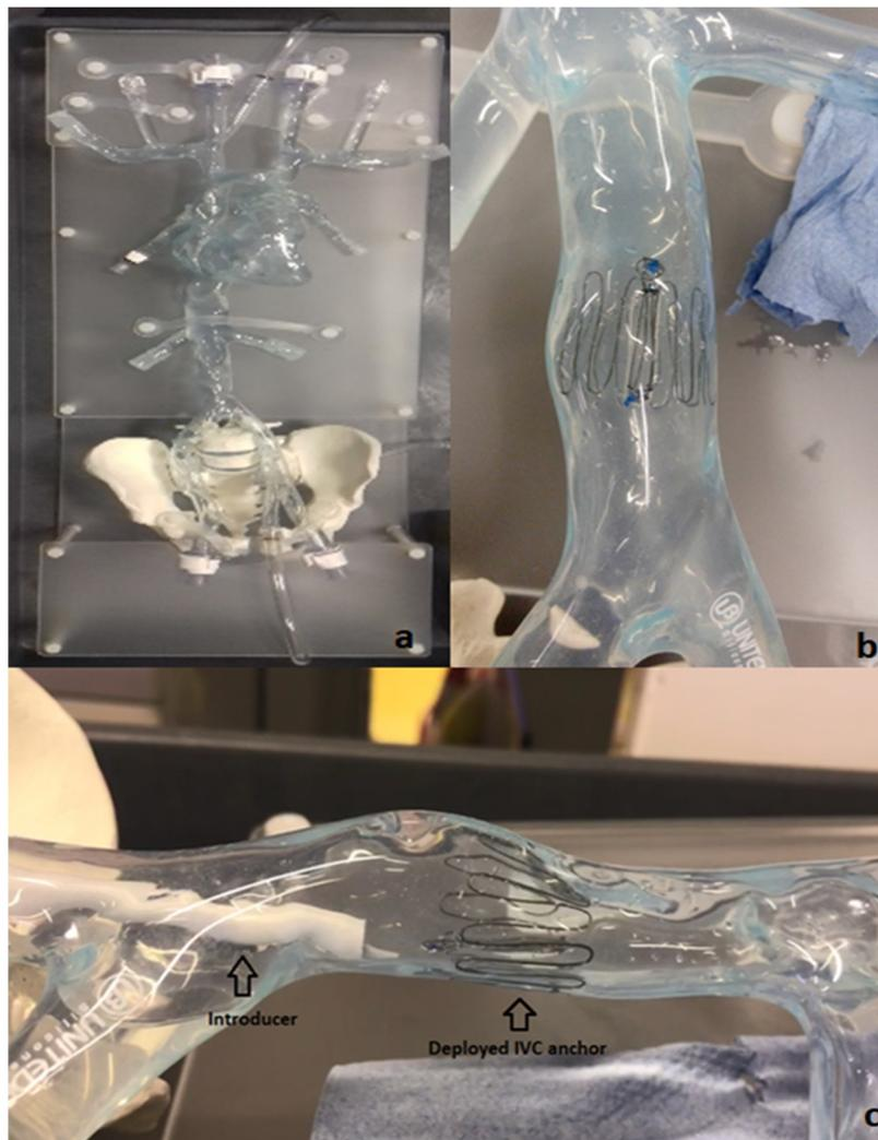
**Figure 4.** Bench model of Vena Cava (a); 10-strut anchor deployed at the target site in the Vena Cava model (b); deployment of the anchor in the bench model using an introducer–dilator as the delivery system (c).
