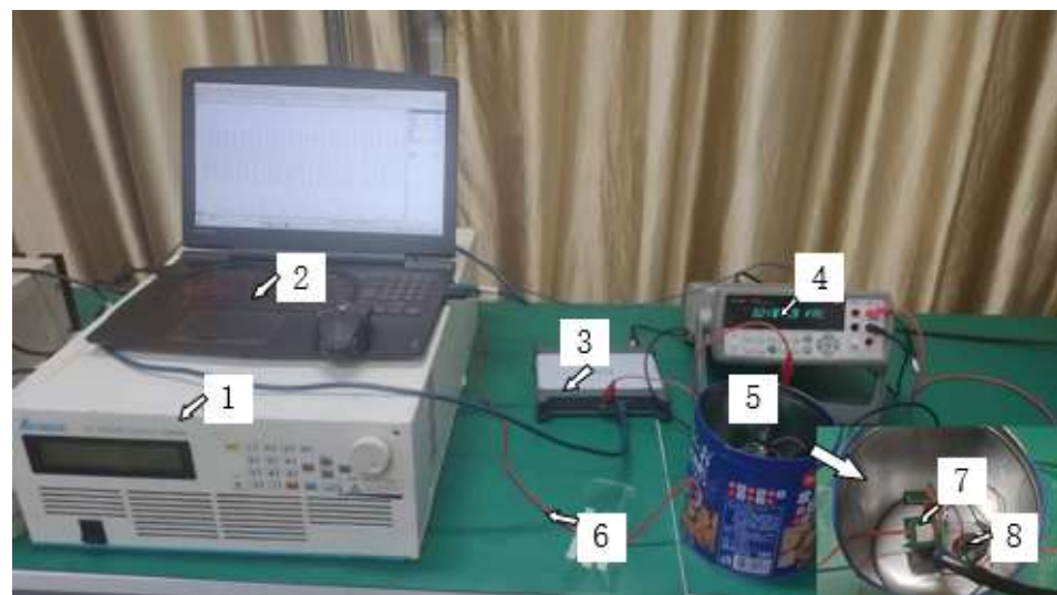
Figure 6. Power frequency experimental platform. (1)—high voltage source, (2)—PC terminal data acquisition, (3)—pico 5443D 16-bit PC oscilloscope, (4)—Agilent 16-bit digital multimeter, (5)—shield cover, (6)—wire to be tested, (7)—sensor, and (8)—9 V dry battery.
