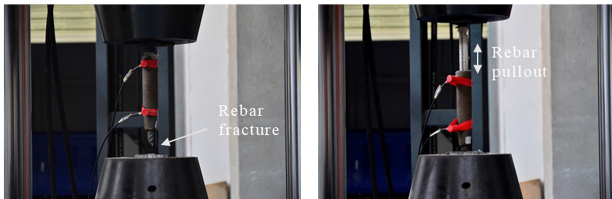
Figure 14. The two typical failure mode of the grouting sleeve connector: (a) rebar fracture; (b) rebar pullout.
