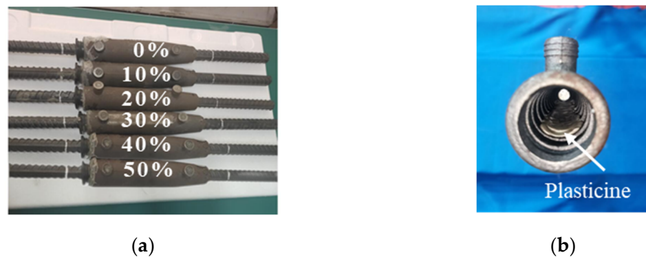
Figure 9. (a) grouting sleeve defect specimen; (b) schematic diagram of internal defects of sleeve.
