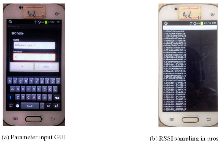
Figure 4. Data acquisition APP. (a) GUI interface for parameter input. (b) RSSI sampling at RP.
