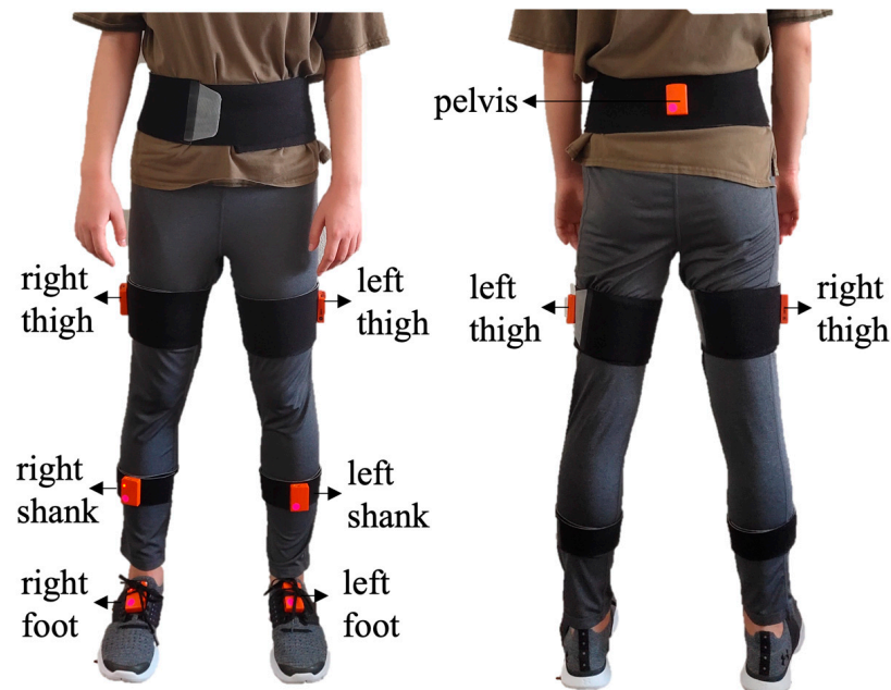
Figure 2. Seven IMU sensors were attached to the lower body.
